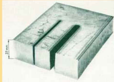
Cutting example from 1964: Comparison of a kerf with conventional torch and a kerf with the first Fine Focus torch (left)
